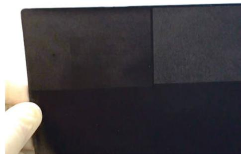
*As we rotate the sample towards the light source, the specular component reflected from the glossiest and smoothest surfaces start increasing, therefore our brain now receives different information from the 3 surfaces. We are shifting to SCE mode.*
