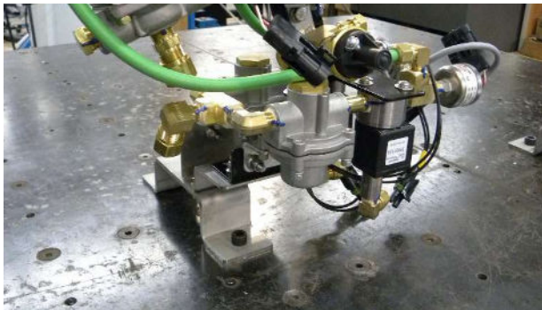
Air brake system - Vibration fatigue test
