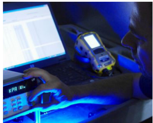
Pressure and electrical computer monitoring while thermal cycling
